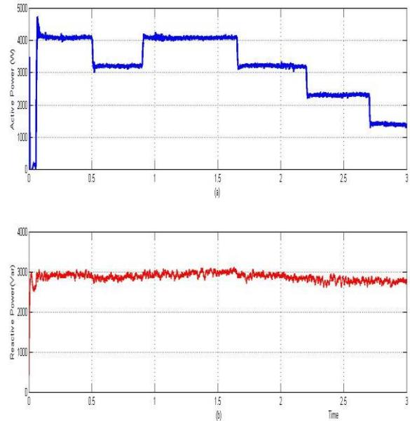
Figure 16 Power Supplied to Grid at Varying Irradiance a) Active power b) Reactive power
