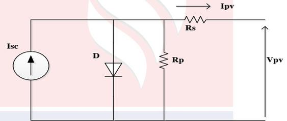
Figure 2 Equivalent Circuit Model of Solar Module
