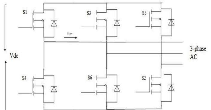
Figure 5 Circuit Diagram of Voltage Source Inverter (VSI)
