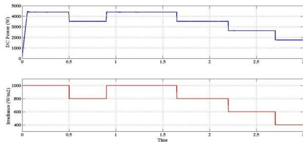
Figure 11 DC Power of Solar PV System at varying irradiance
