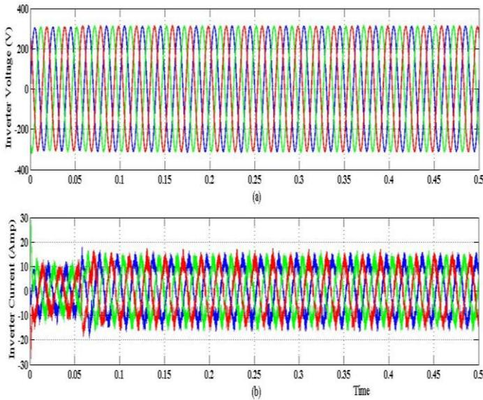
Figure 14 Inverter (a) voltages (b) Current
