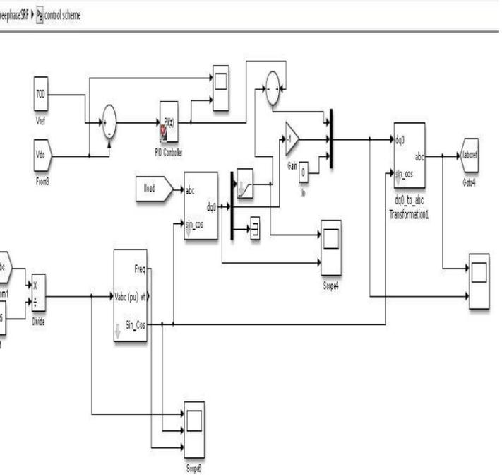
Figure 8 MATLAB Simulation of SRF Control Scheme for Grid Synchronization
