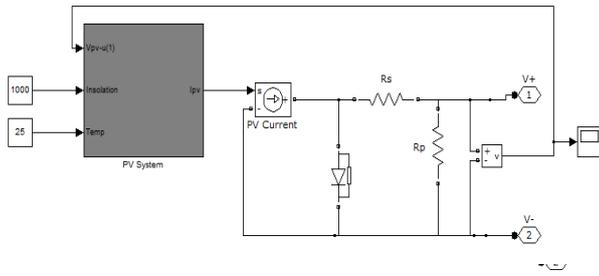
Figure 3 MATLAB Simulation of Solar PV Panel
