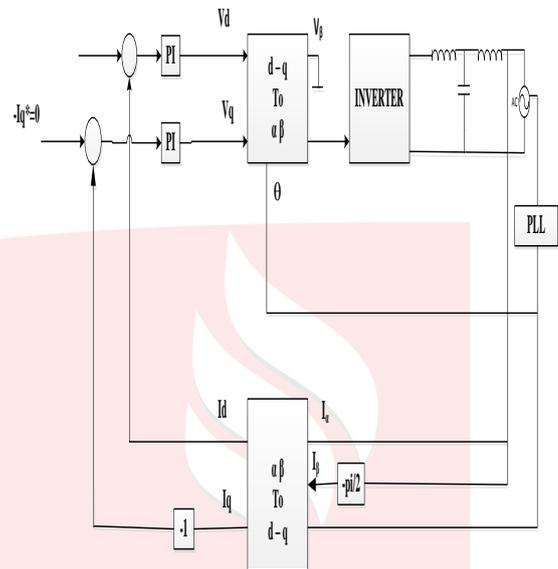
Figure 7 Reference Current Extraction using SRF Theory
