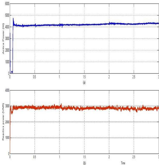
Figure 15 Power supplied to grid at constant irradiance a) Active power b) Reactive power
