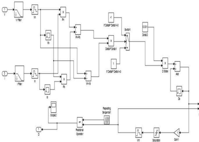
Figure 6 MATLAB Simulation of P&O MPPT Controller
