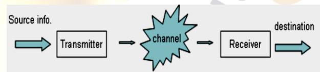
Figure 1.1 Basic elements of communication systems.
