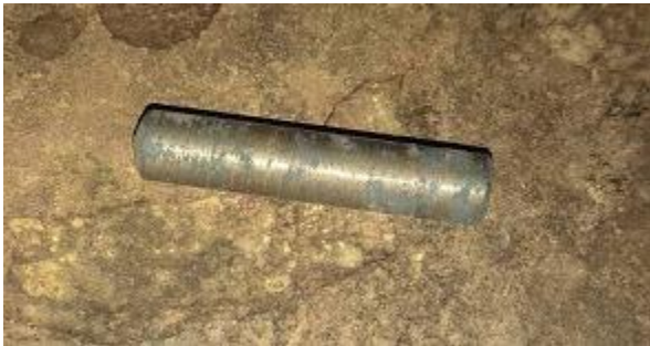
Figure 2 SS410 Sample after Process Annealing
