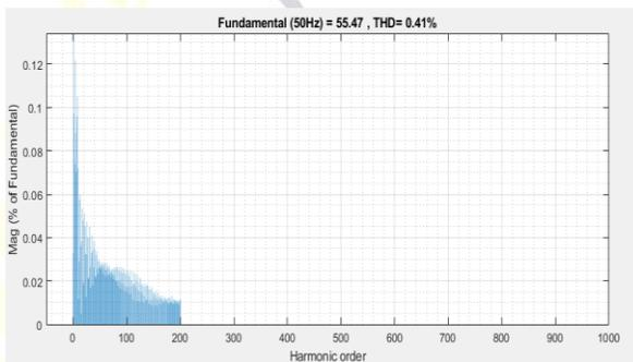
Figure 29: During transient loading, THD percent of current obtained from the load terminal utilizing voltage distortion regulation control
