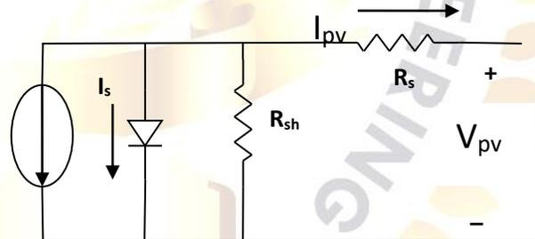
Figure 3 Solar Photovoltaic cell identical circuit
