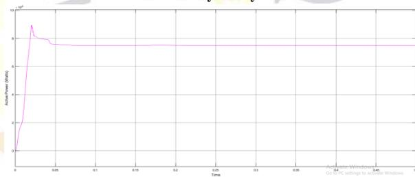
Figure 41: Solar and wind hybrid technology active power production using voltage source controller
