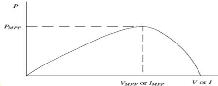
Figure.4 Power curve of a typical Photovoltaic system
