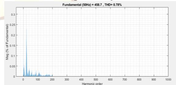
**Figure 12: Voltage distortion modulation regulate for inverter THD percent in voltage of waveform on load terminal**
