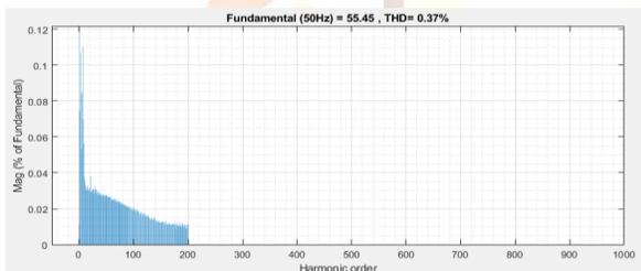
Figure 31: Percentage of THD of the current on load terminal during transient offloading by suggested controller
