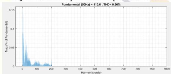
**Figure 21: Percentage of THD in current waveform outcome using recommended DE method for inverter performance improvement control with many objectives**
