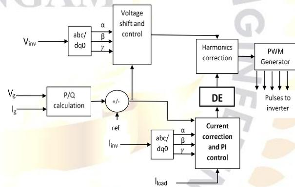
Figure 6: Power Integrated regulator for inverters featuring differential evolutionary (DE) improvement and hysteresis band
