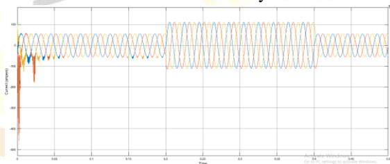
Figure 22: Using voltage distortion modulation control, current is pulled from load terminal.
