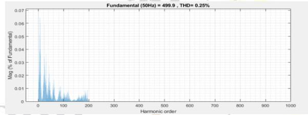
Figure 45: The suggested hybrid solar or wind/fuel cell technology has a THD percent in voltage output.
