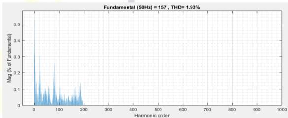
Figure 40: Percentage of THD on current production from solar and wind hybrid system
