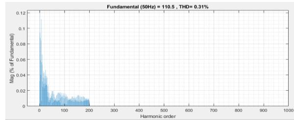
Figure 24: During transient loading, THD percent in current generated from the load terminal employing voltage distortion regulation control
