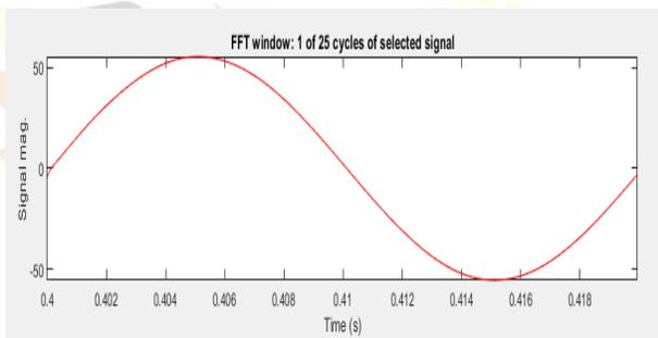
Figure 30: For FFT study of current now at load terminal during transient unloading using the suggested controller
