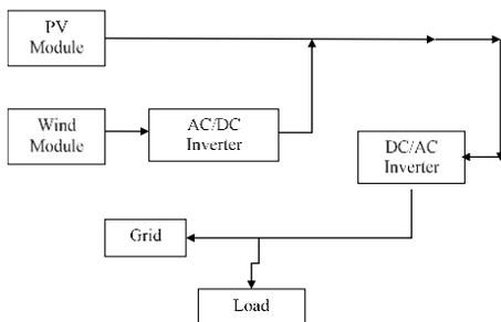
Figure 1: A hybrid energy technology is given and its structure is shown.
