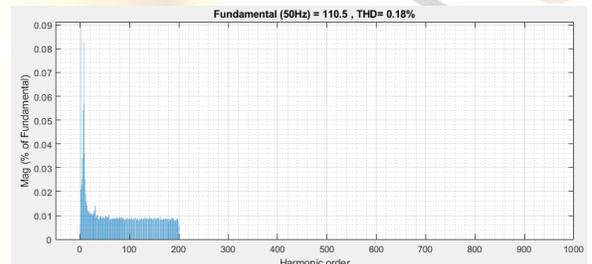
Figure 27: With the suggested controller, THD percent in Current just at Load Terminal at the Time for Transient Loading
