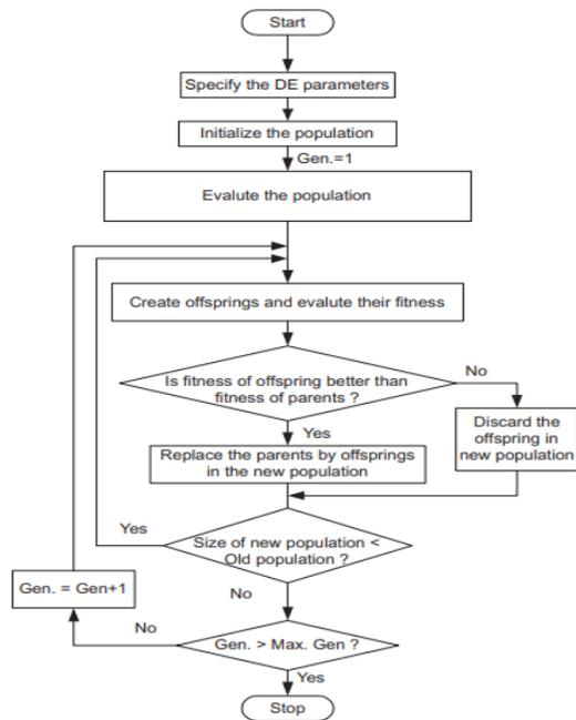
Figure 7: Displays the flow diagram that is Differential Evolutionary Algorithm should be for Converters, which was previously discussed..
