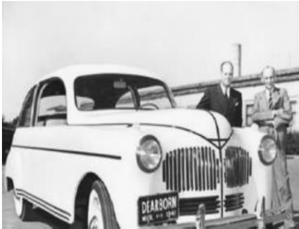
Fig.1. Soy-based composite car. (Lee EC. Bio-based Mater Durable Auto mot Appl2013., n.d.)
