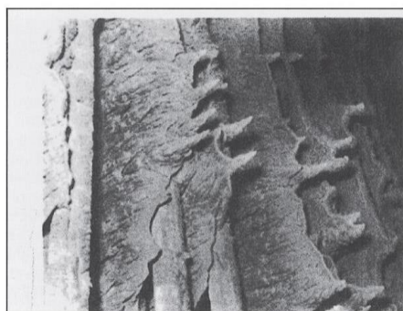
Fig.5: Precipitation fouling of ash particles on super heater tubes [6]
