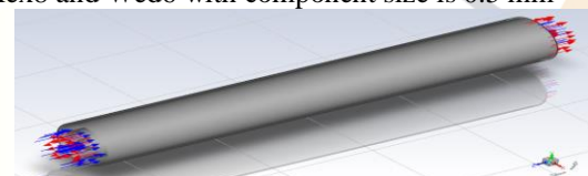
Fig. 8: Concentric tube triple tube heat exchanger with straight baffles of Boundary Condition
