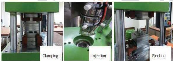
Fig. 2 Different Phases of Injection Molding Process
