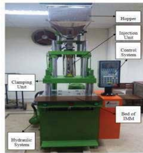
Fig. 1 Vertical plastic injection molding machine
