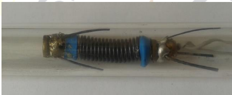
Fig.5 A typical inchworm type robot [4]
