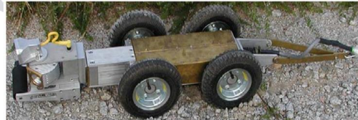
Fig 1 A typical wheeled type in-pipe robot [1]
