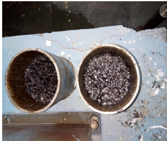
Photo 1 Sample Preparation Marshal Stability Test
