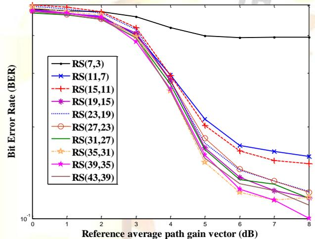
**Fig.3 BER performance of RS codes with constant code rate = 4 under Rician Fading Channel**
