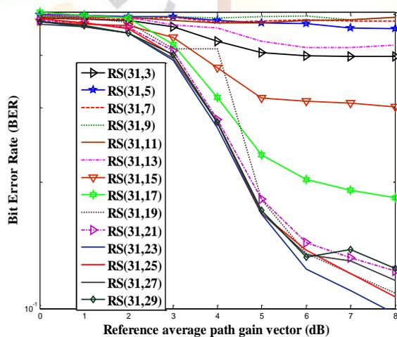
Even though it is similar to previous simulation cases, considerable amount of performance difference exist between the different RS codes. As per this simulation, it is RS(31,23) code that
