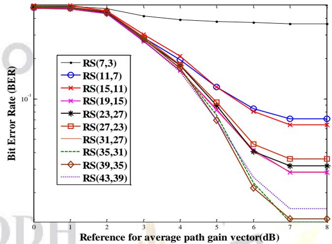
**Fig.2 BER performance of RS codes with constant code rate = 4 under Rayleigh Fading Channel**
