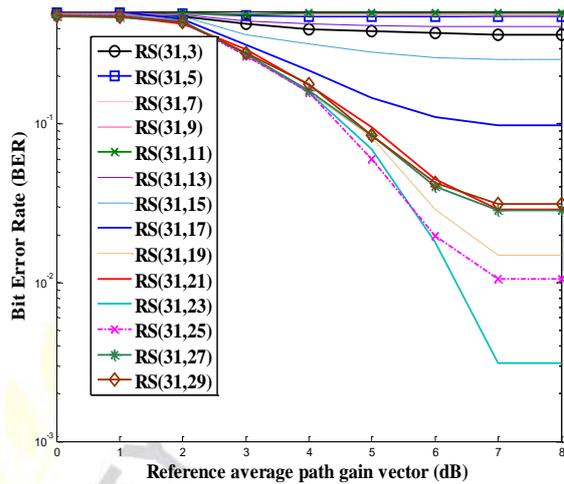
**Fig.4 BER performance of RS codes with constant Galois Field Order = 5 under Rayleigh Fading Channel**
